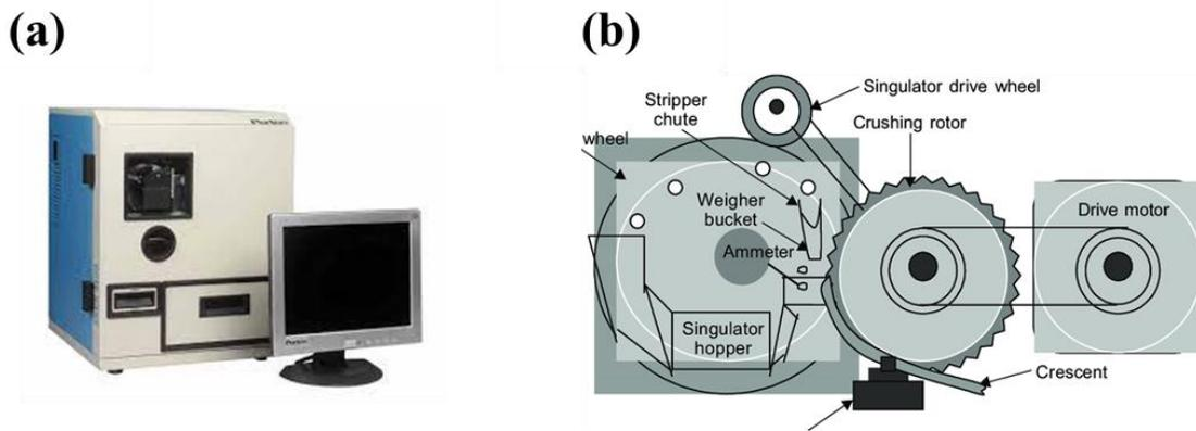
**Figure 1.3** Single Kernel Characterization System (SKCS 4100) (a), SKCS operating mechanisms (b).
