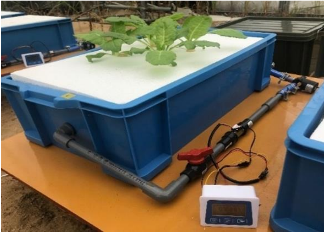
Figure 2-2. The hydroponic system used in this study. The cultivation container dimensions were 620 mm length (L) \times 375 mm width (W) \times 195 mm height (H). The flow inlet and flow outlet were located at the center of the sidewall, and the flow inlet and outlet diameters were both 18 mm.
