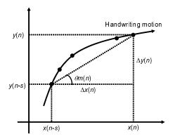
**Fig. 2.** Definition of pen-movement angle  $\theta(n)$ .
