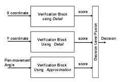
Fig. 5. Proposed multi-matcher verification system.
