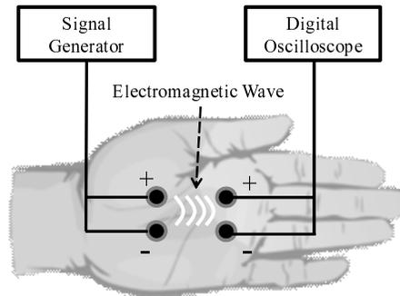
Figure 1. The measuring system of intra-palm propagation signals.
