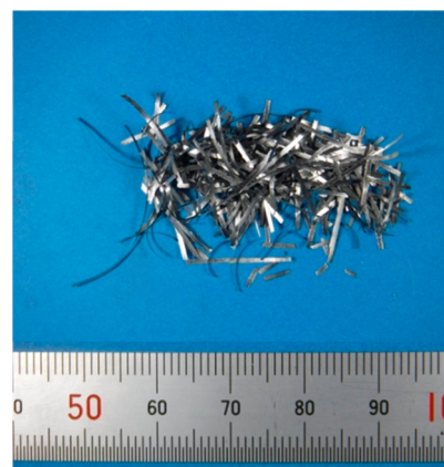
Figure 11. Photograph of the silicide/Si composite ribbon prepared using the rapid quenching method.
