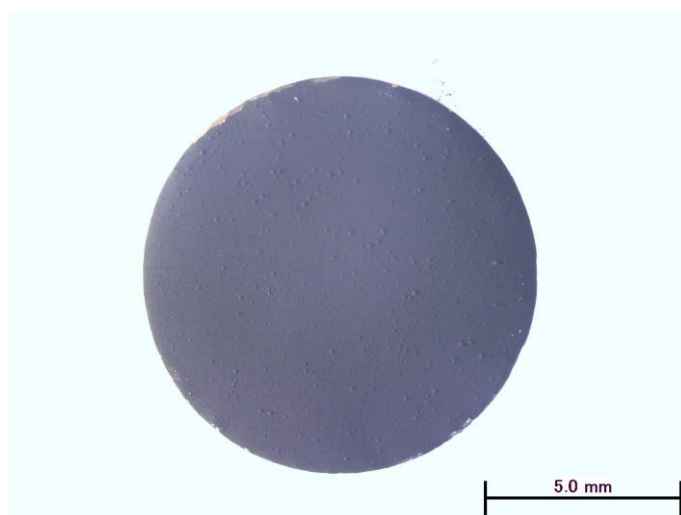
Figure 1-6. Photograph of a fabricated \text{SiO}_x electrode as an example.
