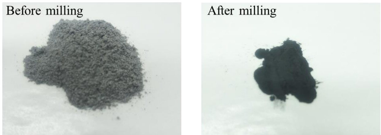
Figure 2-2. Photographs of a mixture of Si, SiO_2 , and Sn powders before MM and 3 wt.% Sn/ SiO_x powder obtained via MM.
