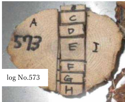
Fig. 2-1-6. Cross-section of logs of Q. serrata used to measure the horizontal distribution of moisture content
